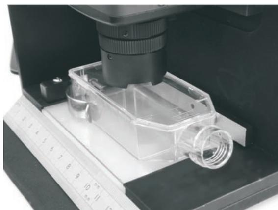
**Figure 2.** The imaging arrangement showing the camera lens, a flask in the jig and the illuminating film below.
